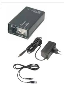
Accubox and connecting cord with cinch- and HEINE-automatic plug. Compact and handy battery box in high-impact polyamid, containing one NiMH rechargeable battery charged by means of a mains transformer. Light in weight and fully-portable, it can be carried in a coat pocket or attached to a belt by a clip.
